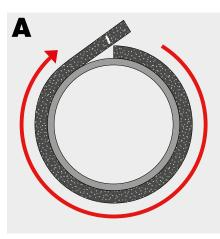
**A)** The measurement is obtained by using a strip of K-FLEX<sup>®</sup> of the same thickness to be used as the insulation. This gives you the measurement of the circumference, including the thickness of the insulating material itself.
