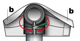
**1)** Place the elastomeric elbow on the piping elbow. Glue the edges of the elastomeric joint with K-FLEX® adhesive.
