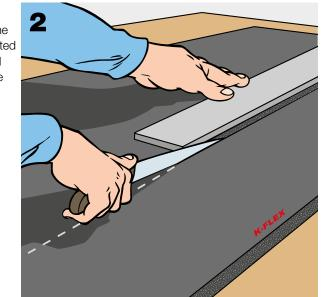
Apply K-FLEX® glue to the surface which has to adhere to the conduit, and to the conduit surface. Use K-FLEX<sup>®</sup> glue to join the edges together. In the example given, for the best results we recommend first to insulate the lower surface of the conduit, then the side walls and lastly the top. This will prevent the penetration of humidity.
