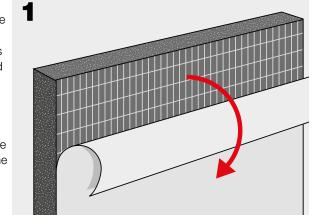
Use K-FLEX<sup>®</sup> glue to join the edges together.
