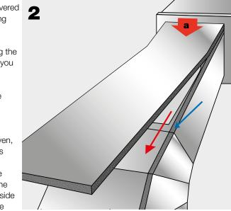
For outdoor applications it is necessary to avoid water stagnation along the horizontal sections for which the material must therefore be installed so as to guarantee a slope of not less than **3° - 5°**
